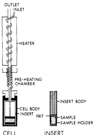
Figure 2. Detail of adsorption cell 5 (Figure 1) showing preheater coil.
